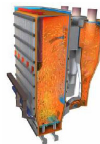
Figure 3. Bubbling fluidized bed furnace [1]
